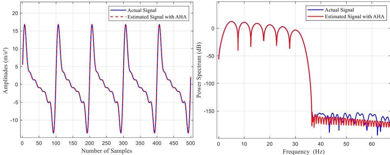
**Figure 3.1.** Test signal and AHA-estimated signal overlap(a). Power spectra of the signals(b).
