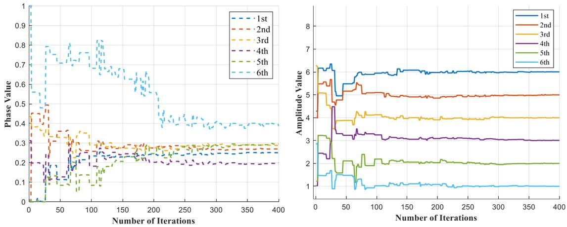
Figure 3.2. Convergence curves of phase (left) and amplitude (right) parameters depending on iterations
