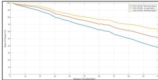
Figure 7. BEV SoC vs. Distance Graph (Acceleration is Exempted)
