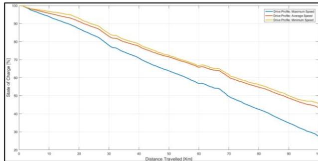
Figure 8. BEV SoC vs. Distance Graph (Acceleration is Included)
