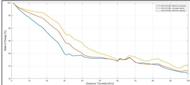
**Figure 5.** HEV SoC vs. Distance Graph (Acceleration is Exempted)
