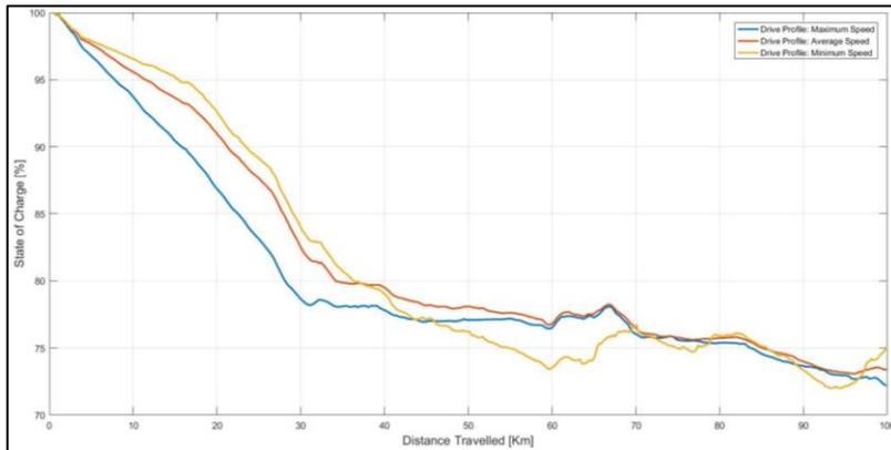
**Figure 6.** HEV SoC vs. Distance Graph (Acceleration is Included)
