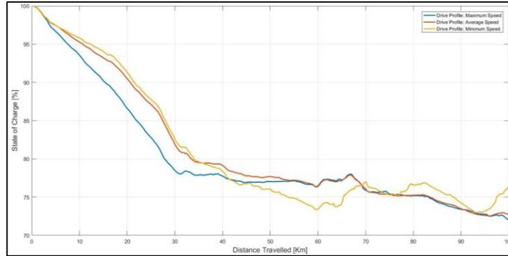
**Figure 9.** HEV SoC vs. Distance Graph (Auxiliary Loads Included)
