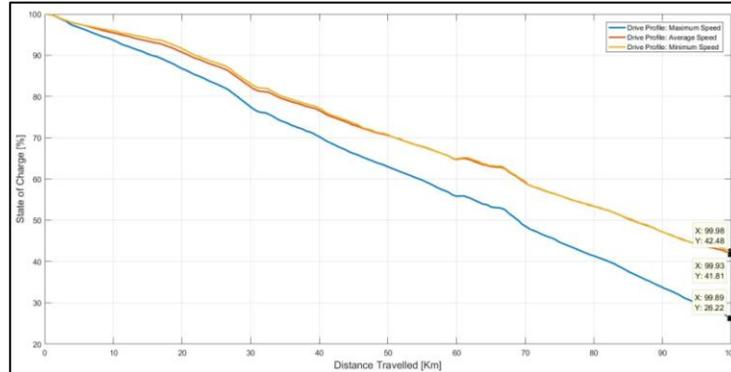
**Figure 8.** BEV SoC vs. Distance Graph (Auxiliary Loads Included)
