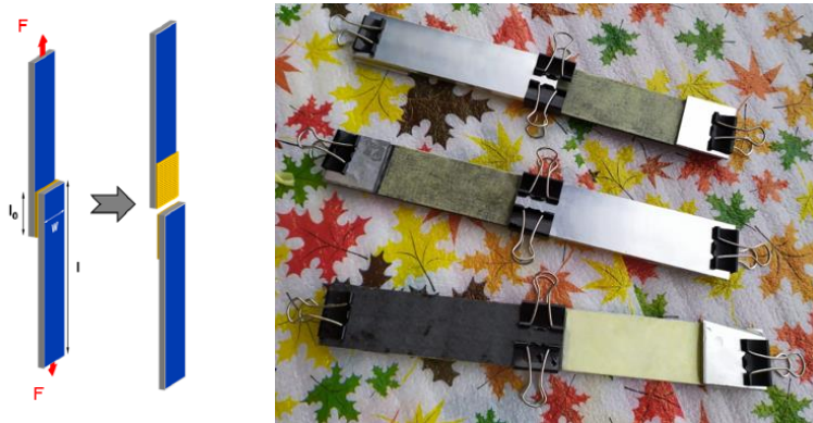
Figure 5. Specimens under tensile lap shear test.
