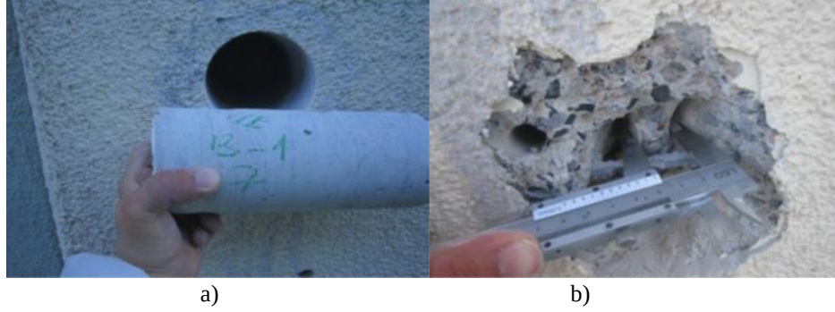
Photo 1: a) Concrete Core sampling, b) Destructive reinforcement detection
